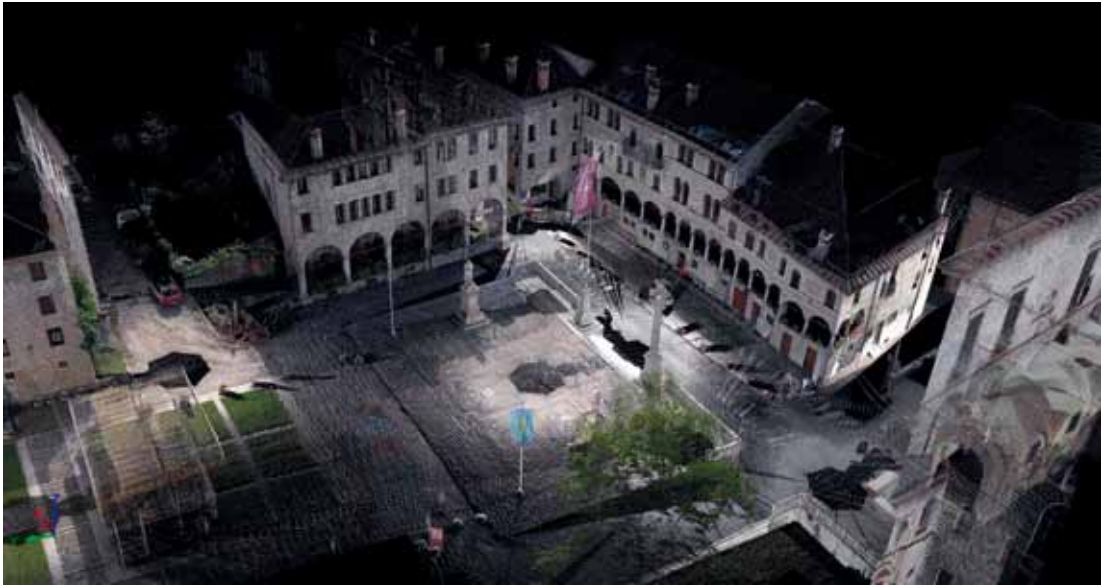
Figure 4 Example of City Model. This is an image derived from a 3D Model of Piazza Vittorio Emanuele, Feltre (Belluno).
