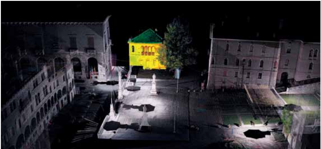
Figure 5 Example of City Model integrated with the thermo camera “ sensing ” data. Piazza Vittorio Emanuele, Feltre (Belluno).
